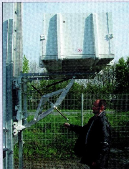
Adjustable turntable height (crank)
