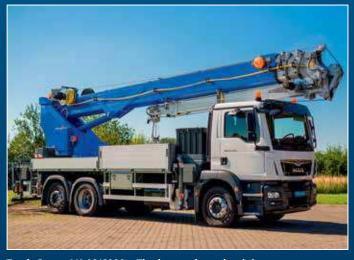
Truck Crane AK 46/6000 - The heavy duty aluminium crane
